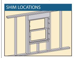
Shims are located uniformly and snugly between the window and the rough opening.
