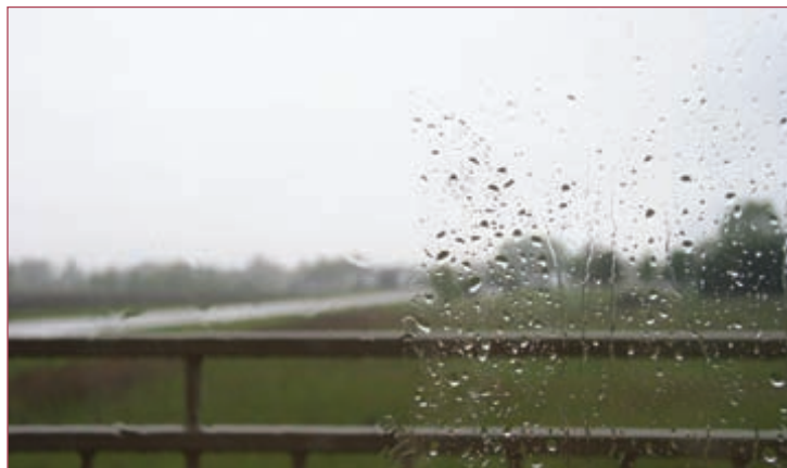
Easy-cleaning window glass (left) versus standard glass (right)
